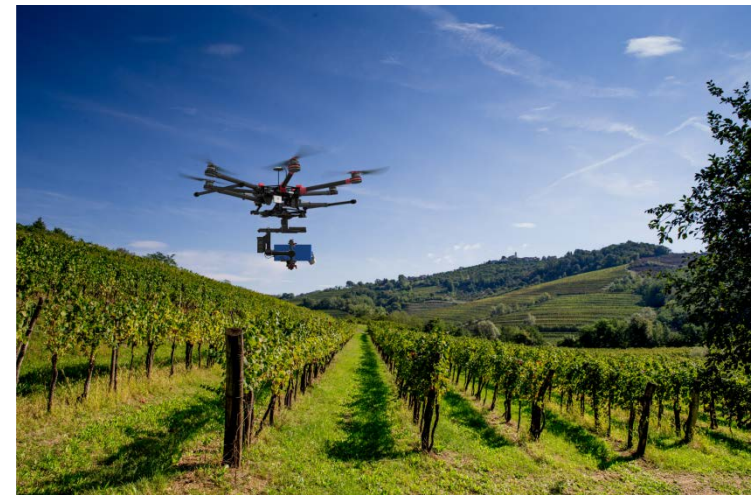
Mock-up of 425 SHARK mounted on DJI Matrice-600 hexa-copter
